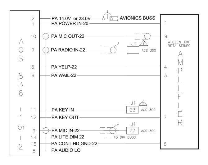
The ACS 836 -1, -2 wiring harness should be constructed of Tefzel aircraft wire (M22759/16 grade). Shielded wires should be used where noted. Adequate protection against wear and chafing should be taken by using a braided cable sleeving or jacket. Before completing installation, verify that all cable connector pins are seated properly and that the connector is securely mounted to the unit mating connector.
