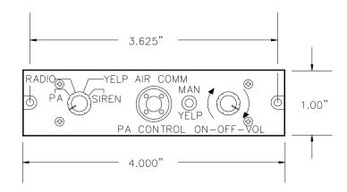
FRONT PANEL WIDTH - 2 HOLE MTG.
