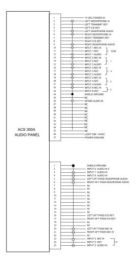
The ACS 300A(SP) wiring harness should be constructed of Tefzel aircraft wire (M22759/16 grade). Power and ground wires should be 18 or 20 AWG, and all other wires may be 22 AWG. Shielded wires should be used where noted. Adequate protection against wear and chafing should be taken by using a braided cable sleeving or jacket. Before completing installation, verify that all cable connector pins are seated properly and that the connector is securely mounted to the unit mating connector.
