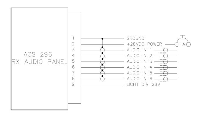
The ACS 296 wiring harness should be constructed of Tefzel aircraft wire (M22759/34 grade). Power and ground wires should be 22 AWG. Shielded wires should be used where noted. Adequate protection against wear and chafing should be taken by using a braided cable sleeving or jacket. Before completing installation, verify that all cable connector pins are seated properly and that the connector is securely mounted to the unit mating connector.
