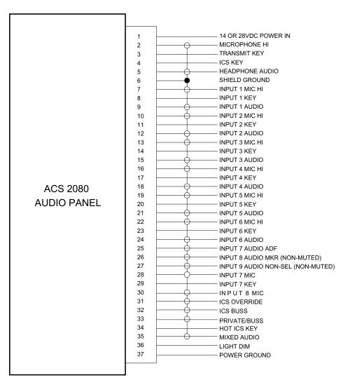
The ACS 2080-300 wiring harness should be constructed of Tefzel aircraft wire (M22759/16 grade). Power and ground wires should be 18 or 20 AWG, and all other wires may be 22 AWG. Shielded wires should be used where noted. Adequate protection against wear and chafing should be taken by using a braided cable sleeving or jacket. Before completing installation, verify that all cable connector pins are seated properly and that the connector is securely mounted to the unit mating connector.
