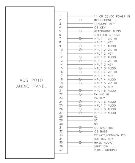
The ACS 2010-300 wiring harness should be constructed of Tefzel aircraft wire (M22759/16 grade). Power and ground wires should be 18 or 20 AWG, and all other wires may be 22 AWG. Shielded wires should be used where noted. Adequate protection against wear and chafing should be taken by using a braided cable sleeving or jacket. Before completing installation, verify that all cable connector pins are seated properly and that the connector is securely mounted to the unit mating connector.
