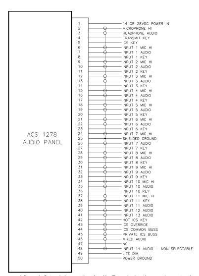
NOTE: Inputs are read from left to right on the Audio Panel plastic overlay, starting on the top row.
