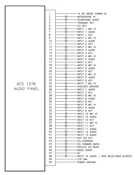
NOTE: Inputs are read from left to right on the Audio Panel plastic overlay, starting on the top row.
