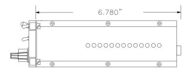
ALLOW UP TO 2.500" FOR REAR CONNECTOR AND CABLE CLEARANCE
